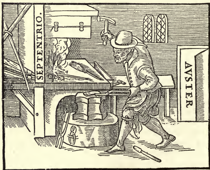
MAGNETIZING HOT IRON BY HAMMERING IT WHILE HELD IN THE MAGNETIC MERIDIAN. 1
